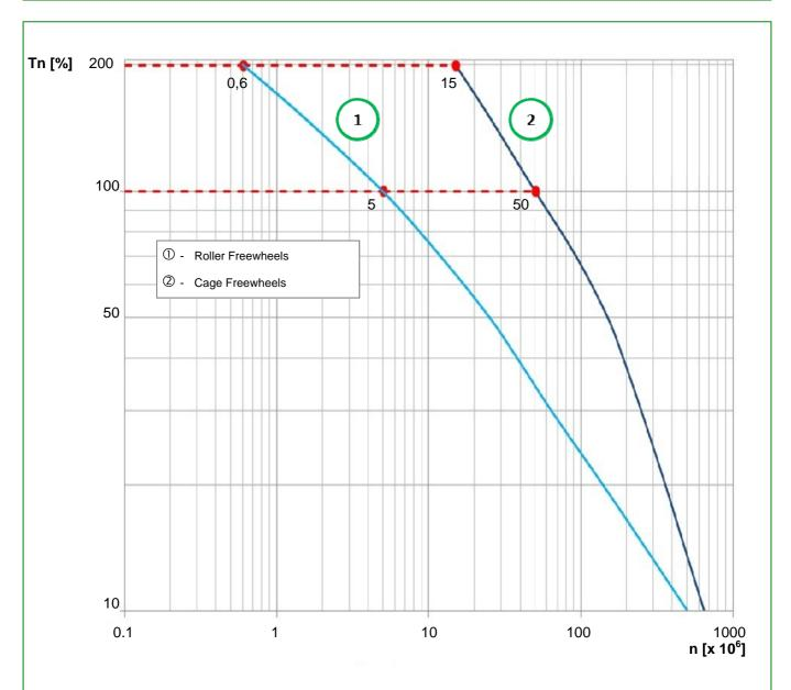
BSM and BSM-G modules are fitted with cage freewheels of the type ② only.
